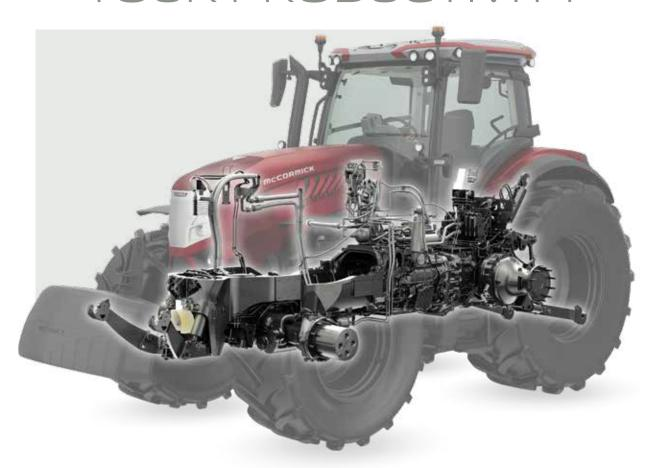
The **X8** tractors feature a closed centre hydraulic system with variable displacement pump. This means that the pump always delivers exactly the quantity of oil that the system requires, thereby eliminating unnecessary power waste. The system supplies 160 l/min to the hitch and remote valves and 115 l/min to the electronic steering system, allowing for simultaneous operation of all hydraulic functions. A pump with up to 212 l/min flow rate is also available to provide high-flow capability.
